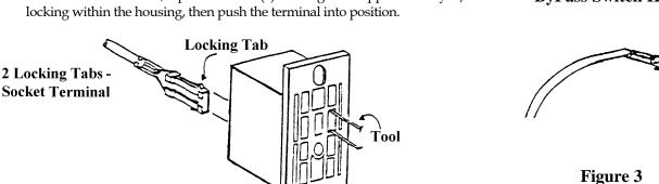
Figure 1 TERMINAL REMOVAL FROM THE MATE-N-LOK PLUGS AND/OR CAPS
